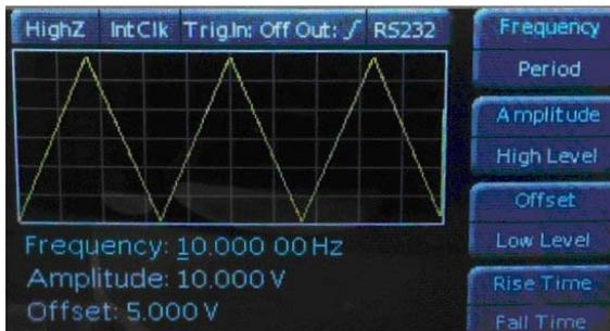
Fig. 8 Triangle wave Y input signal,  $f = 10\text{Hz}$ ,  $U = \pm 5\text{V}$
