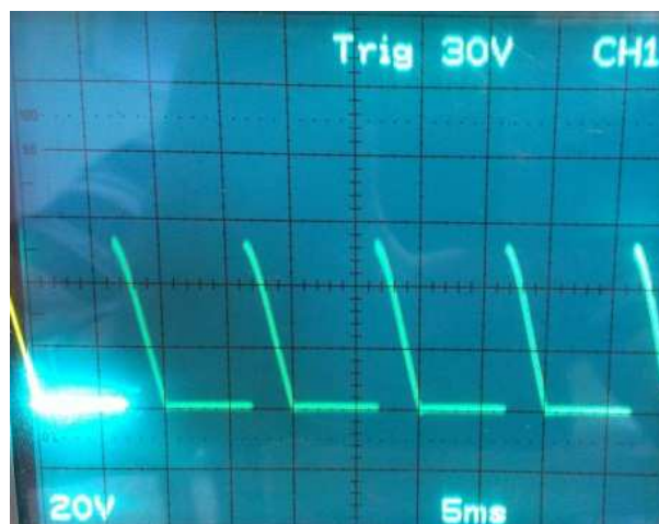
Fig. 8. Output voltage in the case when the control phase angle is 120^\circ and without filtration capacitor
