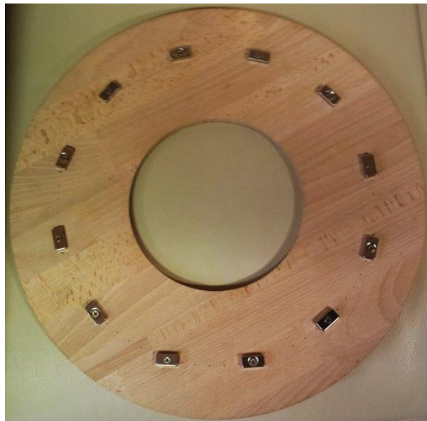
Fig.1 Position of the permanent magnets in the bottom part of the track.
