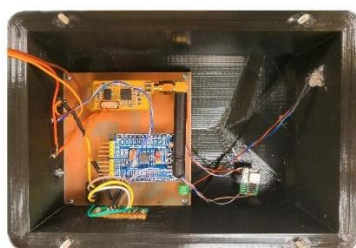
Fig. 8 Displacement of electrical components into base of robotic arm
