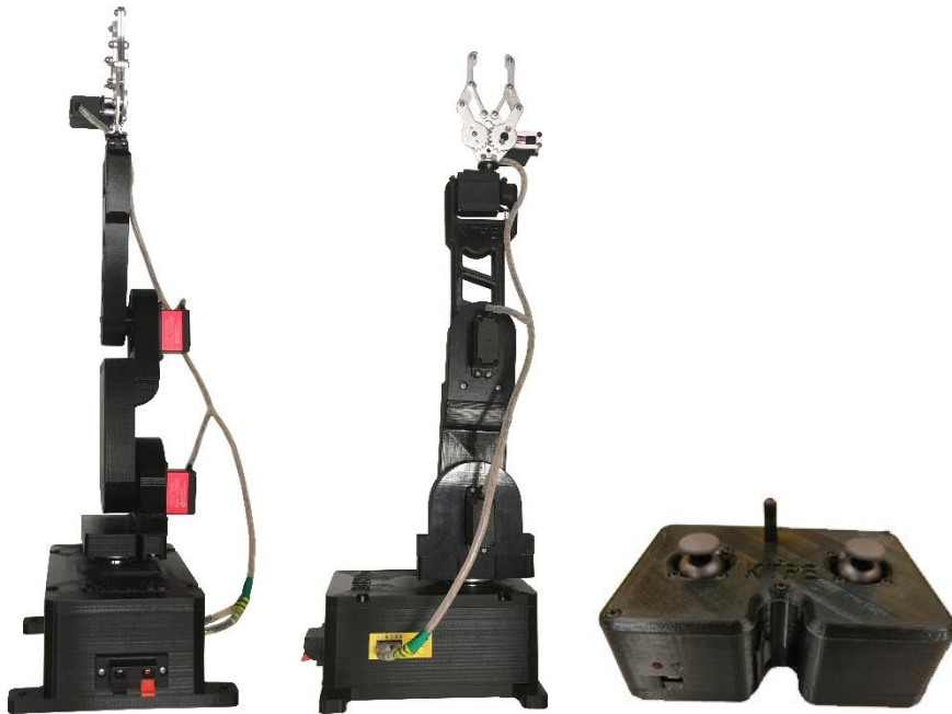
Fig. 12 Constructed all mechanical and electrical parts of the robotic arm and wireless controller
