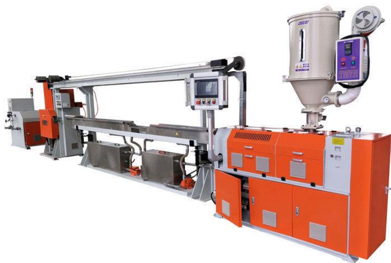
Fig. 1 Commercial manufactured line for production of filament for 3D printers [5]
