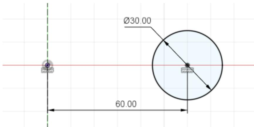
Fig. 1: An example geometry created in Fusion 360 to demonstrate axial symmetry. A circle has been defined which is offset from the z-axis (the dashed line).
