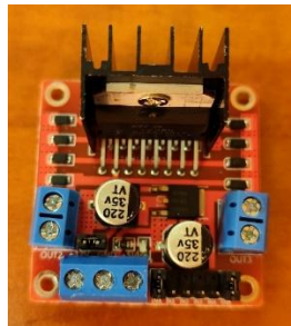
Fig. 10 L298N dual H-bridge motor driver module
