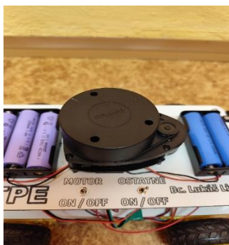
Fig. 11 RPLiDAR A1 sensor mounted on the chassis
