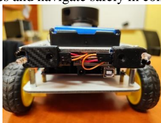
Fig. 12 Infrared proximity sensors (front and rear)
