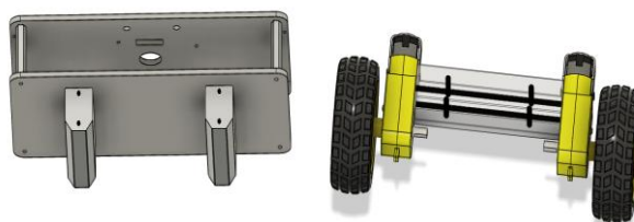
Fig. 3 Motor mounting assembly for the chassis
