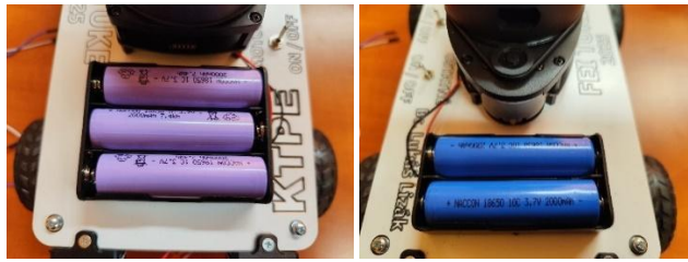
Fig. 8 Power supply configuration with five 3.7 V L18650 batteries
